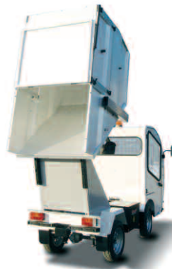
Aluminium cover above container
