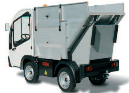
▼ Waste tipping collector
